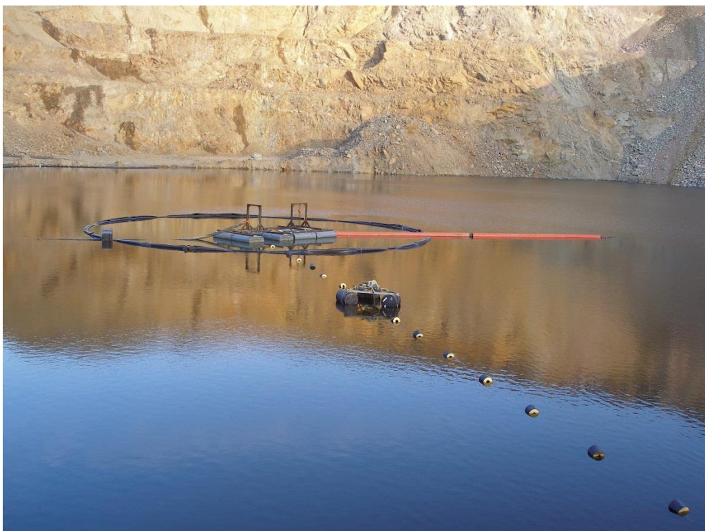
Figure 4: In-situ treatment floating clarifier
